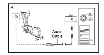
B. Plug one end of the audio cable into the jack beneath the console of the elliptical crosstrainer. Plug the other end of the cable into a 3.5mm Yadapter (available at electronics stores). Plug the Yadapter into the PHONES jack on your computer. Plug your headphones or speakers into the other side of the Y-adapter.
